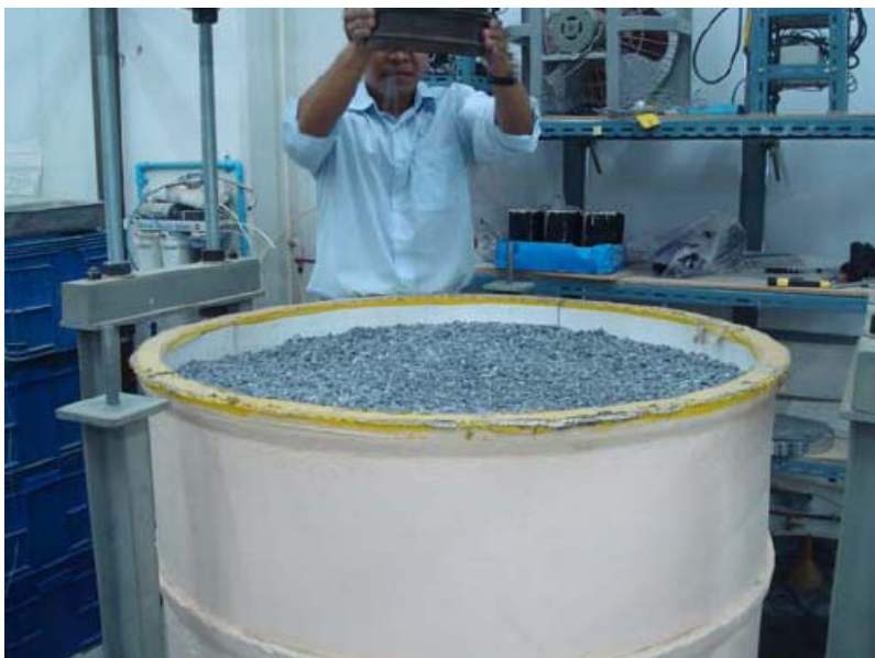
Figure 3.24 Preparation of the modeled gravel layer by sieve opening 1/2 in. (12.5 mm).
