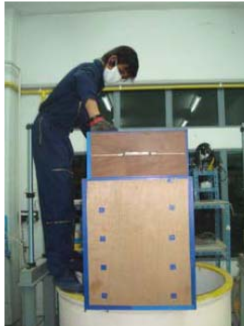
Figure 3.22 Preparation of the modeled subgrade layer by the multiple sieving pluviation apparatus.
