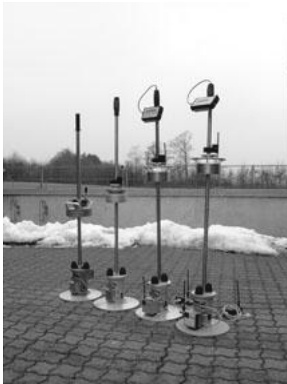
Figure 2.14 Illustration of the Phoenix Falling Weight Deflectometer Model Prima 100
