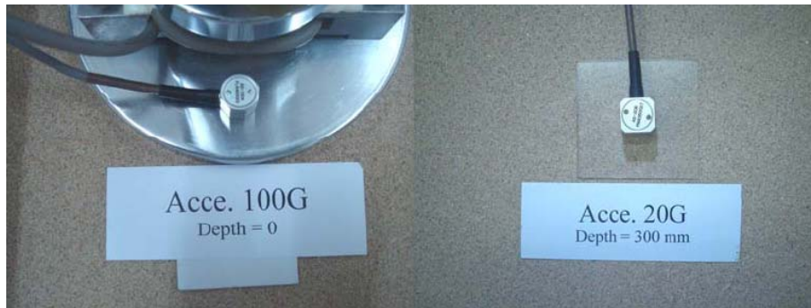
Figure 3.34 Photo showing method to install the accelerometers on the loading plate and inside the ground.
