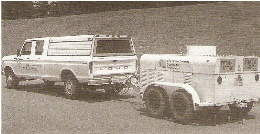
Figure 2.8 Illustration of the Road Rater Model 2008 (after Shahin, 1994).
