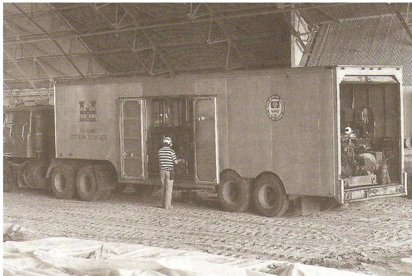
Figure 2.9 Illustration of the WES 16-kip Vibrator (after Shahin, 1994).
