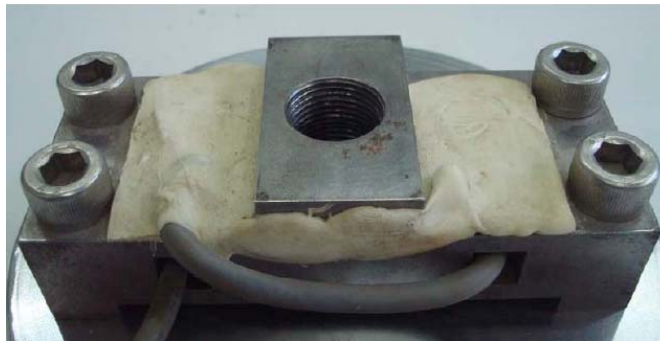
Figure 3.16 Illustration of load cell.
