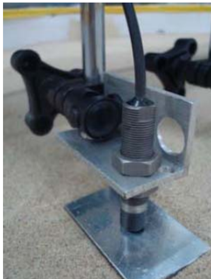
Figure 3.15 Illustration of gap sensor.
