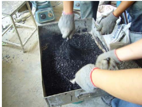
Figure 3.4 Mixing aggregates and asphaltic cement on a tray heated on a store.
